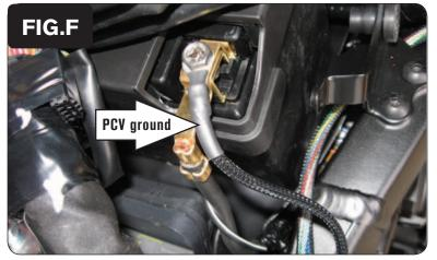
8 Attach the ground wire of the PCV to the negative side of the battery (Fig. F).
