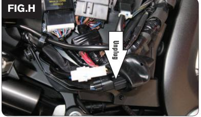
10 Locate the O2 sensor connection under the rubber boot on the right hand side of the bike (Fig. H). Unplug this connection.
