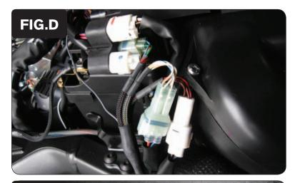
Plug the connectors from the PCV in-line of the stock wiring harness and throttle bodies (Fig. D).
