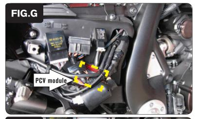
Using the supplied Velcro, secure the PCV to the plastic cover under the right hand side cover (Fig. G). Mount the PCV behind the stock electronics.
