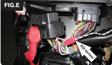
7 Using the supplied Posi-tap attach the GREY wire of the PCV harness to the stock WHITE wire of the small ECU plug (Fig. E).
