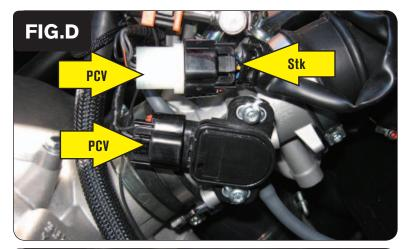
Plug the connectors from the PCV in-line of the stock wiring harness and the TPS (Fig. D).
