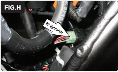
11 Locate the stock O2 sensor connection.
