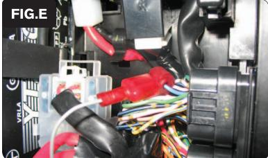
9 Using the supplied posi-tap, attach the GREY wire of the PCV to the BLUE wire on the ECU.
