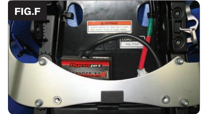
10 Using the supplied Velcro, secure the PCV in the tail section of the bike as shown in Figure F.
