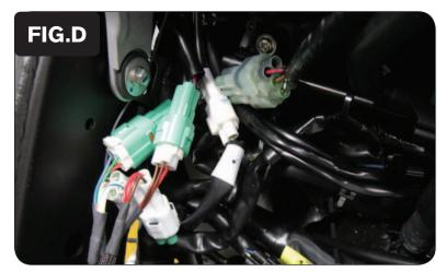
Plug the PCV harness in-line of the stock wiring harness and throttle bodies (Fig. D).
