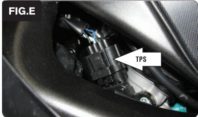
8 Unplug the wiring harness from the Throttle Position Sensor (Fig. E).
