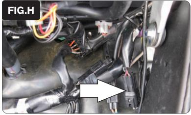
12 Locate the stock O2 sensor connection.
