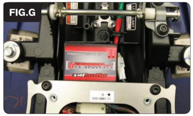
Install the PCV in the tail section using the supplied Velcro, if needed (Fig. G).
