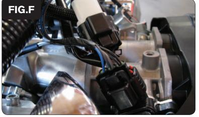
Plug the PCV harness in-line of the stock wiring harness and each fuel injector (Fig. D).
