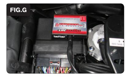
11 Using the supplied Velcro attach the PCV to the top of the ECU (Fig. G).
