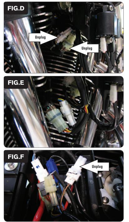
6 Unplug the WHITE 3-pin connector and the CLEAR 6-pin connector (Fig. D).
