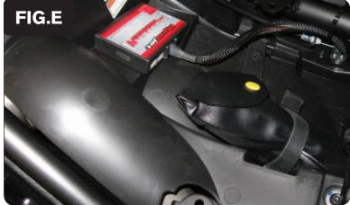
8 Secure the PCV unit in the tail section using the supplied Velcro (Fig. E).
