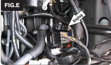
9 Locate the stock O2 sensor in the exhaust. Follow the O2 sensor cable to a connector and unplug it (Fig. E).
