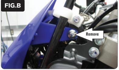
3 Remove the headlight by removing the bolt shown in Figure B on both sides.
