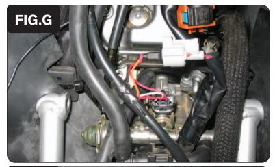
Plug the PCV connectors in-line of the stock wiring harness and injector (Fig. G).
