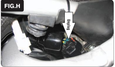
9 Locate the Throttle Position Sensor connector on the right hand side of the throttle body.
