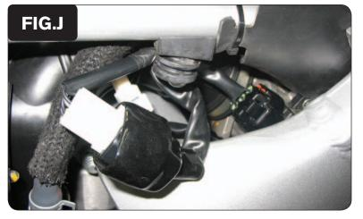
Plug the PCV connectors in-line of the stock TPS and wiring harness (Fig. J).
