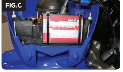
Attach the PCV to the bottom of the headlight using the supplied zip ties (Fig. C).
