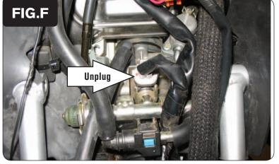
7 Unplug the stock wiring harness from the injector (Fig. F).
