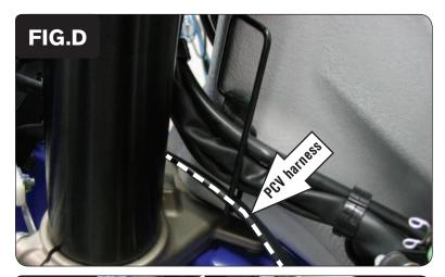
Route the PCV harness thru the cable guide on the left hand side of the frame (Fig. D)
