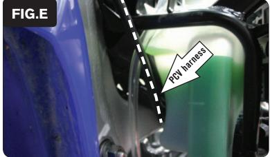
Route the PCV harness between the frame and coolant reserve bottle (Fig. E).
