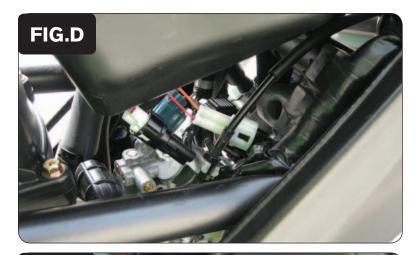
Plug the connectors from the PCV in-line of the stock wiring harness and throttle body (Fig. D).
