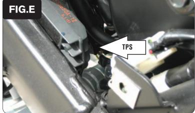
11 Locate the Throttle Position Sensor on the left side of the throttle body. Unplug the TPS connector from the throttle body (Fig. E).
