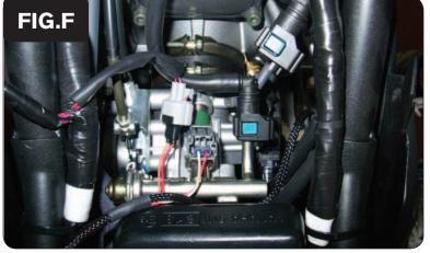
9 Plug the PCV in-line of the fuel injector and the stock wiring harness (Fig. F).
