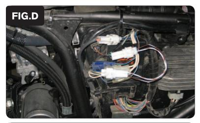
Plug the WHITE 2-pin connectors from the PCV in-line of the stock Crank Position Sensor connectors (Fig. D).
