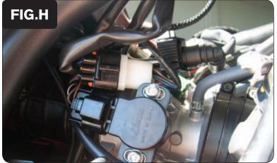
11 Plug the PCV harness in-line of the TPS and stock wiring harness (Fig. H).
