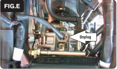
8 Unplug the stock wiring harness from the fuel injector (Fig. E).
