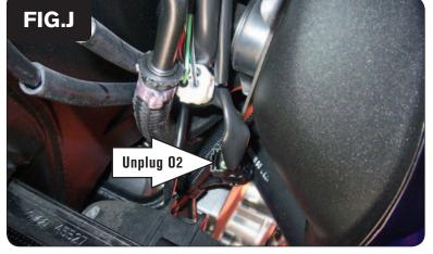
12 Locate the O2 sensor connection. Unplug this connection (Fig. J)
