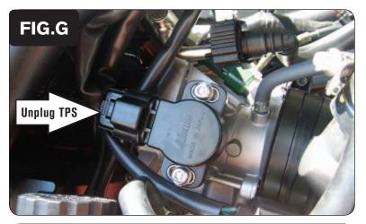
Locate the Throttle Position Sensor on the right side of the throttle body. Unplug the stock wiring harness from the TPS (Fig. G).
