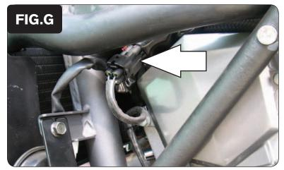
13 Locate the O2 sensor connection (Fig. G). This is a BLACK 4-pin connector located on the left side of the bike near the cylinder head. Unplug the O2 sensor.
