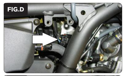
7 Unplug the Throttle Position Sensor from the throttle body (Fig. D).
