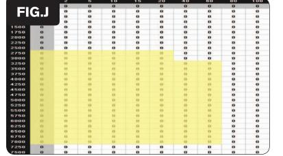
The O2 Optimizer for this model controls the stock closed loop area. This area is represented by the highlighted cells shown in Figure J. The O2 Optimizer is designed to achieve a target AFR of 13.6:1. To use this O2 Optimizer you must retain your stock O2 sensor (even if using Auto-tune).
