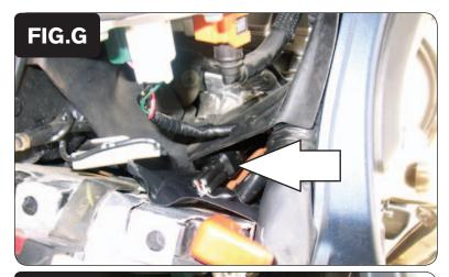
Locate the O2 sensor connection in front of the battery (Fig. G). This is a BLACK 4-pin connector. Unplug the O2 sensor.
