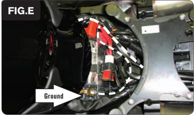
9 Attach the ground wire from the PCV to the negative side of the battery (Fig. E).
