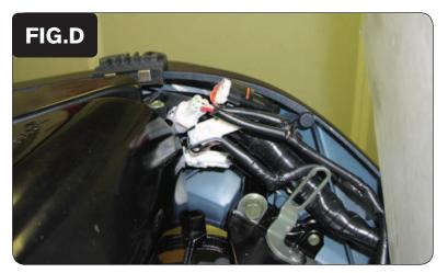
8 Plug the connectors from the PCV in-line of the stock wiring harness (Fig. D).
