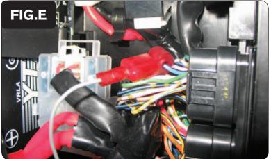
7 Using the supplied posi-tap attach the GREY wire of the PCV to the BLUE wire of the ECU (Fig. E).
