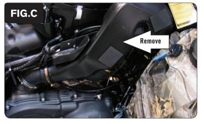
Remove the intake tube for the CVT clutch on the right hand side of the quad (Fig. C).
