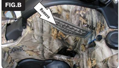
3 Remove the right hand side cover (Fig. B) and the same cover on the left side.
