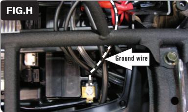
12 Attach the ground wire from the PCV to the negative side of the battery (Fig. H).
