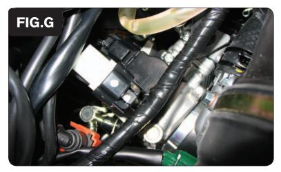
Plug the wiring harness from the PCV in-line of the stock wiring harness and TPS (Fig. G).
