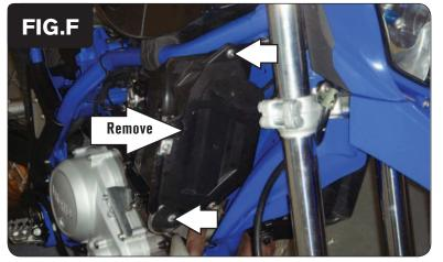
9 Locate and remove the battery box cover. This is located at the front, right side of the bike (Fig F).
