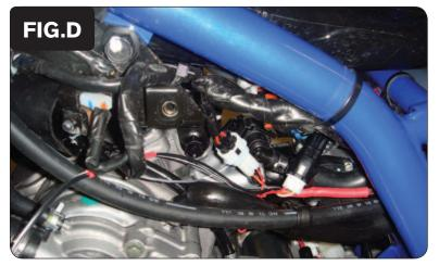
6 Plug the connectors from the PCV in-line with the stock wiring harness (Fig D).
