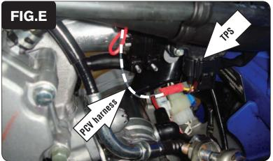
7 Locate the 5-pin BLACK Throttle Position Sensor connector on the left hand side of the throttle body (Fig E).
