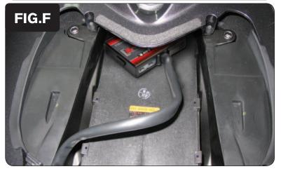
8 Using the supplied Posi-tap, secure the GREY wire from the PCV to the WHITE wire of the ECU as shown in Figure D.
