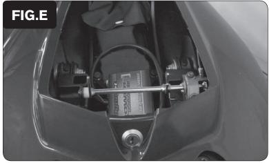
12 Using the supplied Velcro, secure the PCV in the rear section of the trunk as shown in Figure E.
