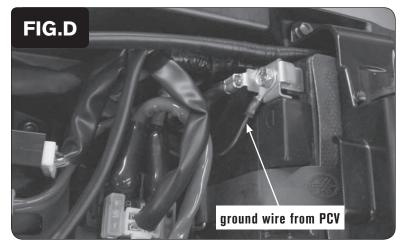
11 Attach the ground wire from the PCV to the negative side of the battery as shown in Figure D.
