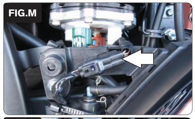
16 Locate the stock O2 sensor connection under the right hand side cover and unplug this connection (Fig. M)
