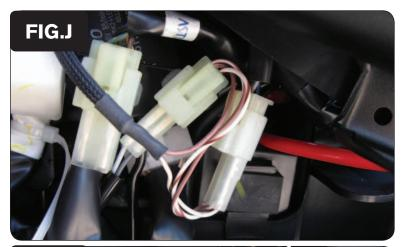
13 Plug the PCV harness in-line of the stock crank sensor and wiring harness (Fig. J).
