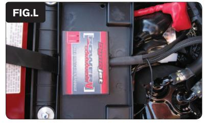
Using the supplied Velcro, secure the PCV to the tray on top of the battery (Fig. L).
