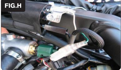
11 Plug the PCV harness in-line of the stock wiring harness and coil (Fig. H).
