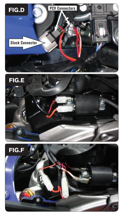
7 Plug the PCV wiring harness in-line with the fuel injector and stock wiring harness (Fig. D).
