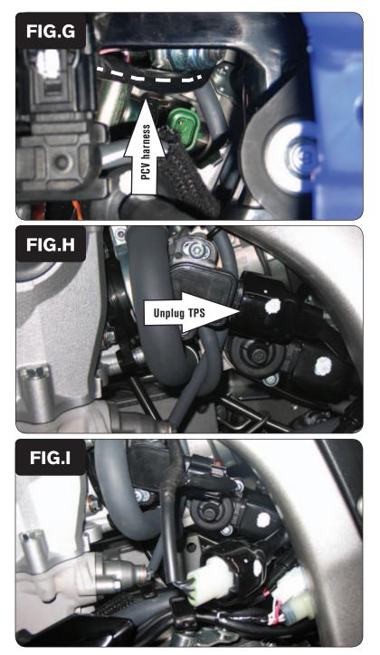
13 Route the set of 3 pin connectors, and the set of 2 pin connectors, of the PCV harness down the left side of the throttle body (Fig. G).
