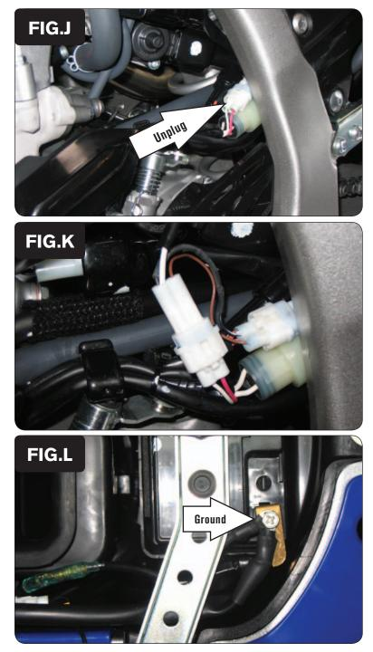
16 Unplug the Crank Position Sensor connectors on the left side of the quad behind the frame rail (Fig J).
