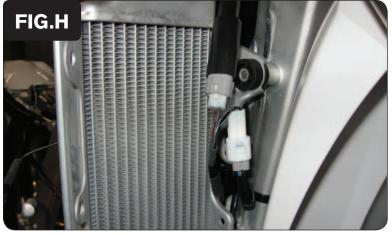
12 Plug the PCV harness in-line of the stock wiring harness for the Throttle Position Sensor connectors (Fig. H).
