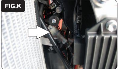
Locate the ignition coil connectors behind the radiator on the left hand side of the bike (Fig. K).
