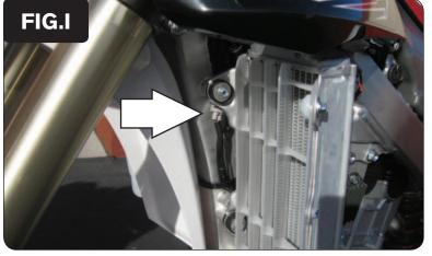
Locate the crank position sensor connector on the front of the radiator left of the frame (Fig I).
