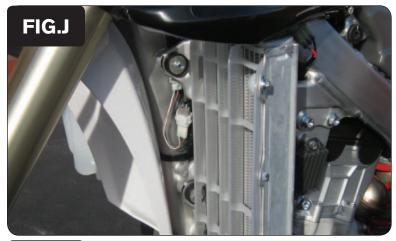
Plug the PCV harness in-line of the stock wiring harness for the crank position sensor connectors (Fig. J).
