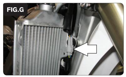
11 Locate the 3 pin GREY connector and unplug it (Fig. G).
