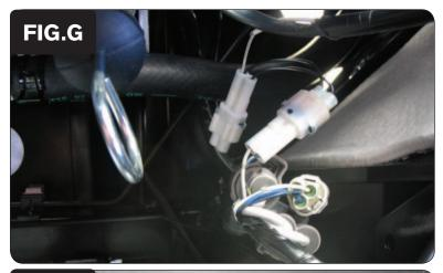
10 Plug the PCV connectors in-line of the stock crank pickup coil and wiring harness (Fig. G).
