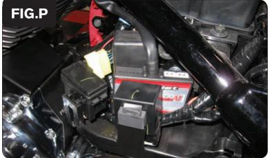
Secure the PCV under the left hand side cover using the supplied Velcro (Fig. P).
