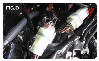
Plug the connectors from the PCV in-line of the stock wiring harness and the throttle bodies (Fig. D).
