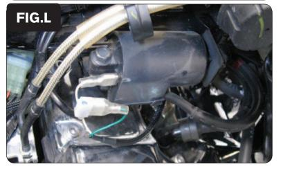
Plug the pair of GREEN colored wires from the PCV in-line of the ignition coil and the stock GREY/RED wire (Fig. L).
