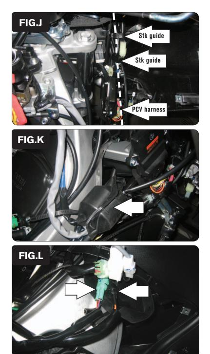
16 Route the fuel side of the PCV harness down the right side following the stock wiring harness.
