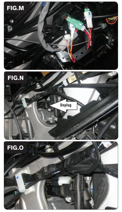
19 Plug the PCV connectors in line with the stock injector connectors (Fig. M). The PCV ORANGE wires go to the GREEN connector for cylinder #1. The PCV YELLOW wires go to the BLACK connector for cylinder #2.
