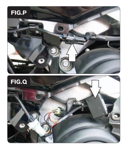
24 Locate the stock O2 sensor connection and unplug it.
