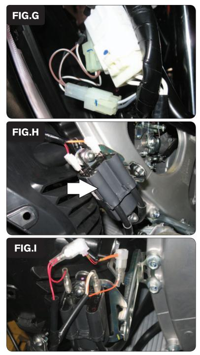
12 Plug the PCV in-line of the stock crank pick-up coil connectors (Fig. G).
