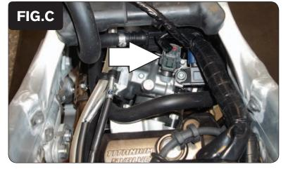
5 Locate and unplug the stock wiring harness from the fuel injector on top of the bike's throttle body (Fig. C).
