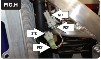
10 Plug the PCV wiring harness in-line of the stock wiring harness and CPS (Fig. H).
