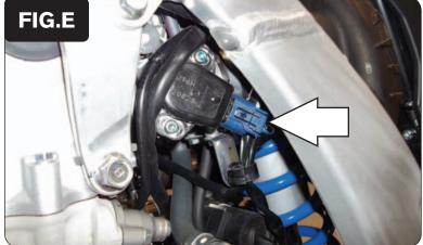
7 Locate and unplug the stock wiring harness from the bike's Throttle Position Sensor (Fig. E).
