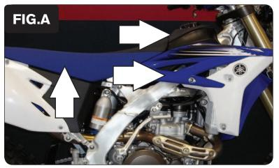
1 Remove the seat, the radiator side covers, and the fuel tank (Fig. A).
