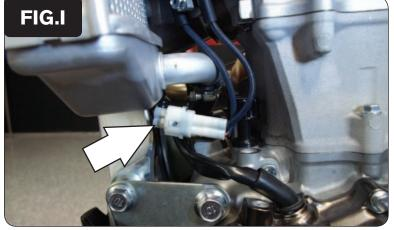
11 Locate and unplug the stock wiring harness from the bike's Ignition Coil (Fig. I).
