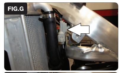
9 Locate and unplug the stock wiring harness from the bike's Crank Position Sensor (Fig. G).
