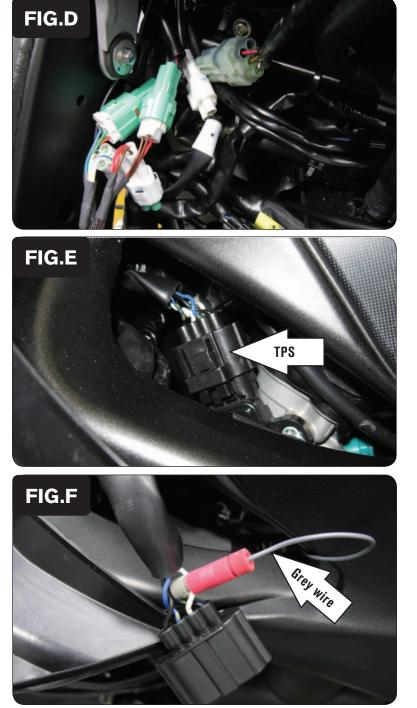
7 Plug the PCV harness in-line of the stock wiring harness and throttle bodies (Fig. D).
