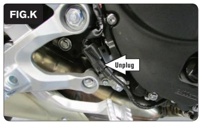
Locate and unplug the stock connector for the bike's stock O2 sensor (Fig. K).
