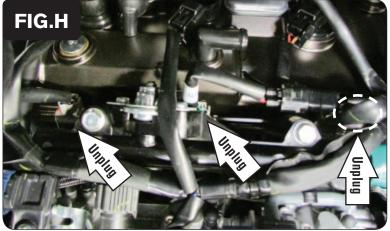
Unplug the stock wiring harness from all three of the bike's Fuel Injectors (Fig. H).
