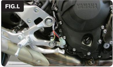
Plug the supplied O2 Optimizer in-line of the stock O2 sensor connectors (Fig. L).
