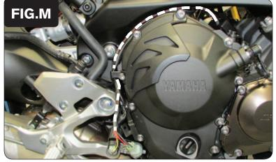
17 Route the O2 Optimizer wiring harness along-side the stock wiring up the back of the engine towards the top of the gear box (Fig. M).
