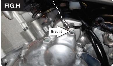
Secure the PCV ground wire with the ring lug to the engine case bolt shown in Figure H on the right side of the engine.
