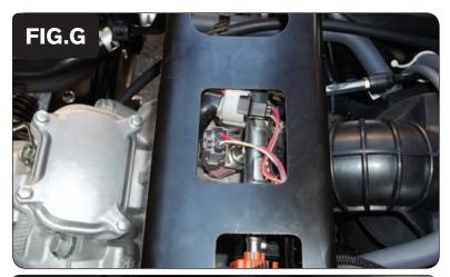
12 Plug the pair of 2-pin connectors from the PCV wiring harness in-line of the fuel injector and the stock connector (Fig. G).
