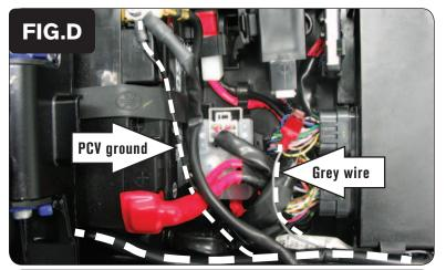
Attach the ground wire from the PCV to the negative (-) terminal of the bike's battery, as shown in Figure D.
