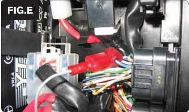
9 Using the supplied posi-tap, attach the GREY wire of the PCV to the BLUE wire on the ECU.
