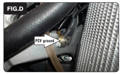
7 Secure the PCV ground wire with the ring lug to the common ground located on the frame just below the PCV module mounting location (Fig. D).
