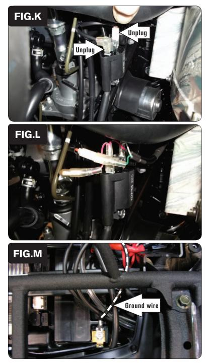
14 Locate the ignition coil on the right side of the quad, forward of the engine; and unplug the 2 stock coil wires (Fig. K).
