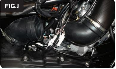
11 Plug the wiring harness from the PCV in-line of the stock wiring harness and TPS (Fig. G).
