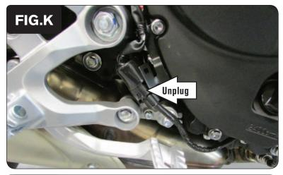
Locate and unplug the stock connector for the bike's stock O2 sensor (Fig. K).
