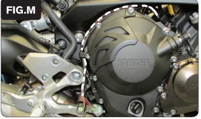
17 Route the O2 Optimizer wiring harness along-side the stock wiring up the back of the engine towards the top of the gear box (Fig. M).
