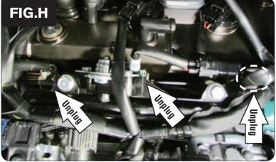
Unplug the stock wiring harness from all three of the bike's Fuel Injectors (Fig. H).
