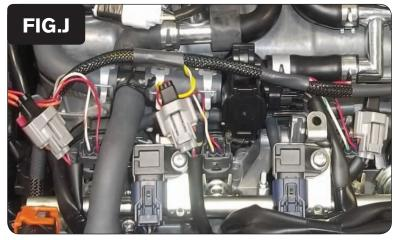
14 Plug the PCV wiring harness in-line of each Fuel Injector and the stock wiring harness (Fig. J).
