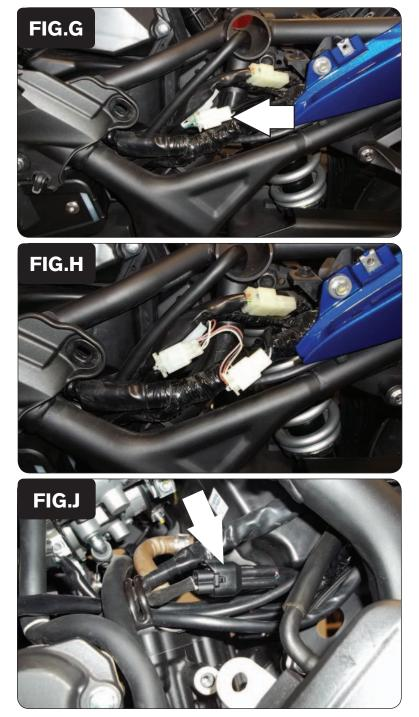
9 Unplug the crank position sensor connector (Fig. G). This is a CLEAR, 3 pin connector on the left side of the motorcycle.
