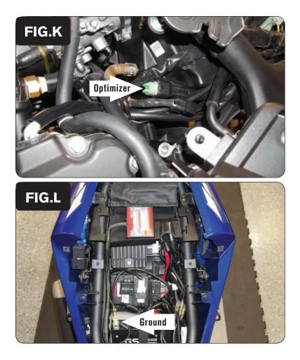
12 Plug the O2 Optimizer into the stock wiring harness (Fig. K).
