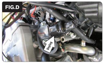
5 Unplug the Throttle Position Sensor at the rear of the throttle bodies (Fig. D).
