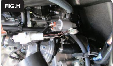
Plug the PCV wiring harness in-line of the stock Crank Position Sensor connectors (Fig. H).
