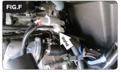
7 Unplug the stock Crank Position Sensor connectors (Fig. F).
