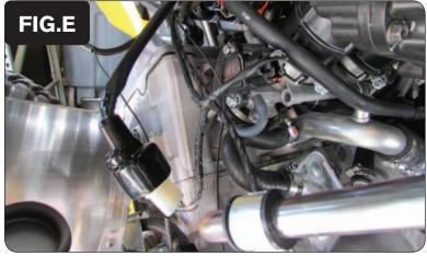
6 Plug the PCV wiring harness in-line of the TPS and the stock wiring harness (Fig. E).
