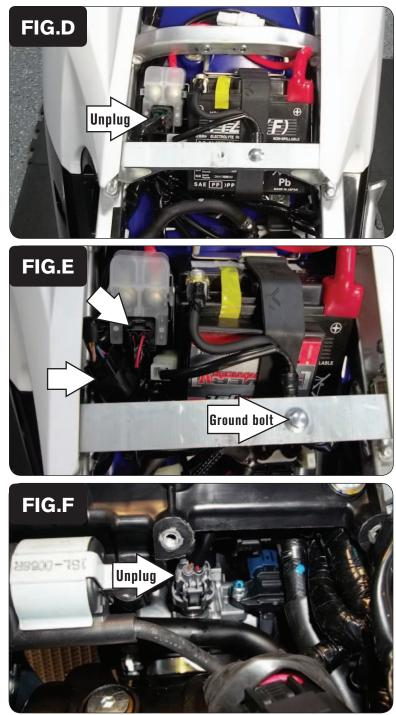
5 Unplug the stock wiring harness from the bike's starter solenoid just right of the battery (Fig. D).
