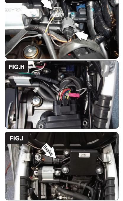
11 Plug the PCV wiring harness in-line of the Fuel Injector and the stock wiring harness (Fig. G).
