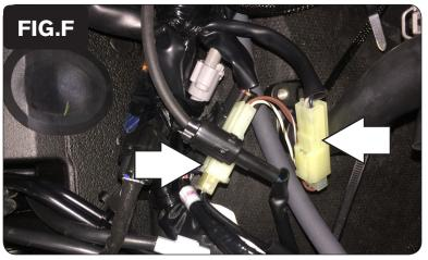
10 Unplug the crank position sensor connector.
