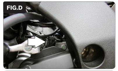
Plug the PCV in-line of the stock gear position sensor and wiring harness (Fig. D).
