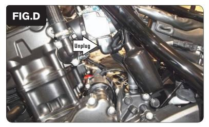
9 On the left hand side of the throttle bodies, unplug the Throttle Position Sensor (Fig. D).
