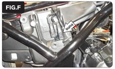
12 Unplug the stock O2 sensor connectors located behind the right sidecover (Fig. F).
