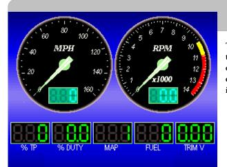
The Dual Analog Gauges screen allows you to view real time data or play back a saved log file. This screen can only be viewed when the Dual Analog Gauges box is checked. Refer to "Gauge Setup" on page 5 for more information.
