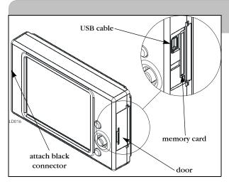
The Dynojet LCD Display allows you to view real time Power Commander data, log data being displayed, and store and send maps to the Power Commander on the fly. The Display provides the following information from the Power Commander: throttle position, duty cycle, current map, and fuel change. The Display can provide more information by adding the Expansion Hub (boost, speed, and gear) or the Ignition Module (ignition change).
