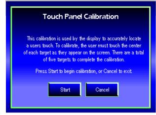
Touch Panel Calibration allows you to calibrate the touch screen should it become unusable. This is done before the Display is shipped, but may need to be performed by the user in the future.
