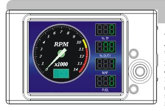
The Display is designed with touch screen capabilities. All menus and information can be accessed by touching the screen.
