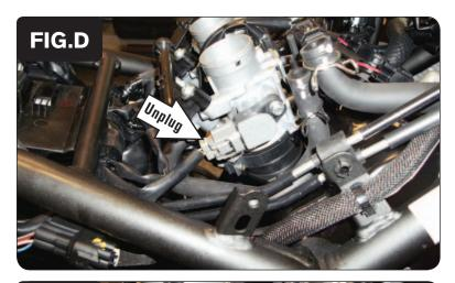
7 Locate and unplug the Throttle Position Sensor on the right hand side of the throttle bodies (Fig. D).
