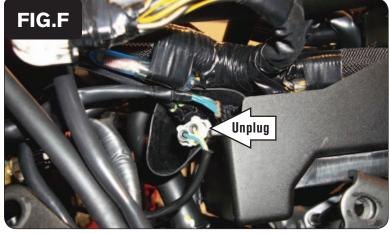
9 Locate and unplug the stock Crank Position Sensor connectors (Fig. F).
