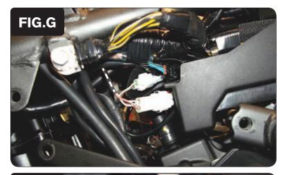
10 Plug the PCV wiring harness in-line of the stock Crank Position Sensor connectors (Fig. G).
