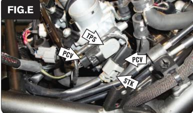
Plug the connectors from the PCV wiring harness in-line of the TPS and the stock wiring harness (Fig. E).
