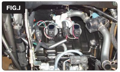
12 Plug the PCV wiring harness in-line of the stock wiring harness and the Ignition Coils (Fig. J).
