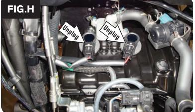
At the top of the engine, unplug the stock wiring harness from both of the Ignition Coils (Fig. H).
