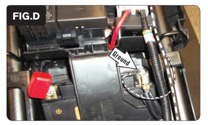
Secure the PCV ground wire with the small ring lug to the negative (-) terminal of the bike's battery (Fig. D).
