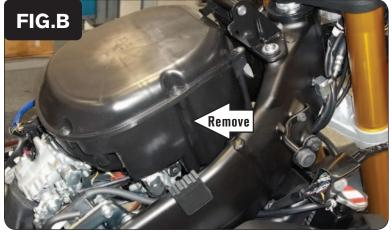
2 Remove the airbox (Fig. B).
