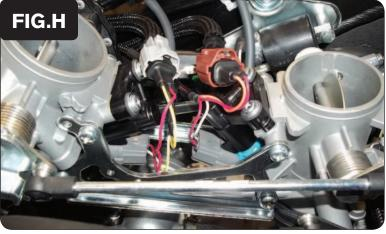
8 Locate and unplug the stock Fuel Injectors, which are located between the throttle bodies (Fig. G).
