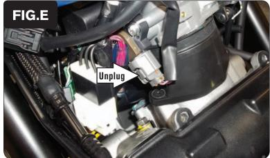
On the left side of the rear cylinder throttle body, locate and unplug the bike's lower primary Throttle Position Sensor (Fig. E).
