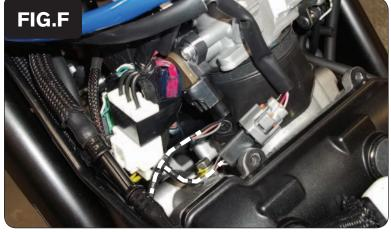
Plug the pair of the 3-pin connectors on the PCV wiring harness in-line of the bike's TPS and the stock wiring harness (Fig. F).
