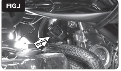
Unplug the stock wiring harness from the front fuel injector (Fig. J).
