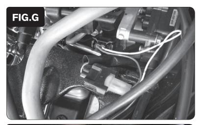
10 Plug the YELLOW colored wires from the PCV in-line of the rear fuel injector and the stock wiring harness (Fig. G).
