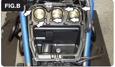
3 Remove the airbox by removing the 6 bolts shown in Figure B.
