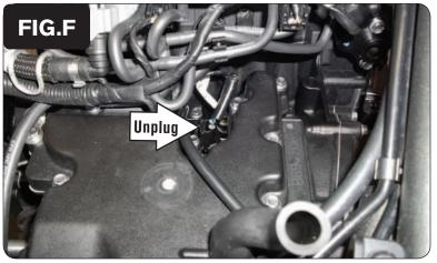
9 Unplug the Crank Position Sensor connector (Fig. F).
