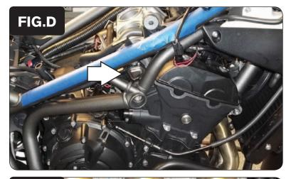
6 Unplug the Throttle Position Sensor connector from the throttle bodies (Fig. D).
