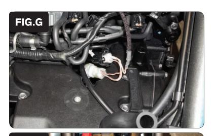
10 Plug the PCV wiring harness in-line of the CPS and the stock wiring harness (Fig. G).
