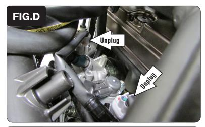
7 Unplug the stock wiring harness from both Fuel Injectors (Fig. D).
