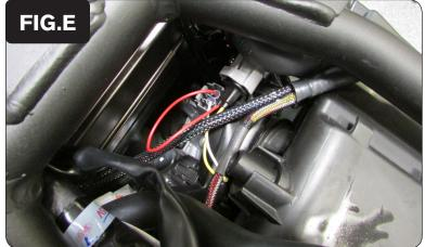
Plug the PCV wiring harness in-line of the Fuel Injectors and the stock wiring harness (Fig. E).
