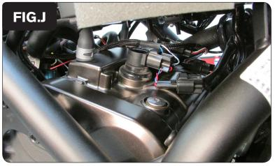
13 Plug the PCV wiring harness in-line of the Ignition Coils and the stock wiring harness (Fig. J).
