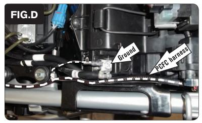
Secure the PCFC ground wire with the small ring lug to the negative (-) terminal of the bike's battery (Fig. D).
