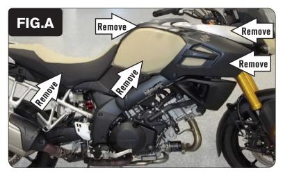
1 Remove the seat, the body panels surrounding the fuel tank, and remove the fuel tank (Fig. A).
