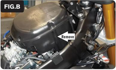
2 Remove the airbox (Fig. B).
