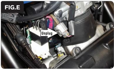
On the left side of the rear cylinder throttle body, locate and unplug the bike's Throttle Position Sensor (Fig. E).
