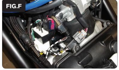
Plug the pair of the 3-pin connectors on the PCFC wiring harness in-line of the bike's TPS and the stock wiring harness (Fig. F).
