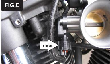
9 Locate and unplug the stock Throttle Position Sensor (TPS) connector as shown in Figure E.
