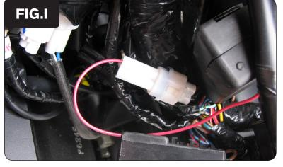
Attach the connector with the red wire from the PCFC to the stock wiring harness as shown in Figure I.
