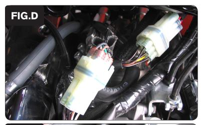
Attach the connectors from the PCFC to the stock wiring harness and the throttle bodies as shown in Figure D.
