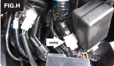
Locate the white 2-pin connector that is taped to the main wiring harness behind the left hand side cover.
