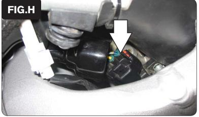
12 Locate the Throttle Position Sensor (TPS) connector.
