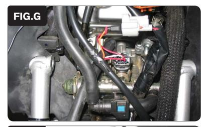
11 Attach the connectors from the PCFC to the stock injector and the stock wiring harness as shown in Figure G.
