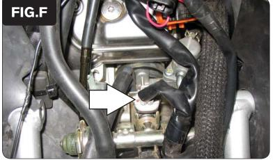
0 Unplug the stock wiring harness from the injector as shown in Figure F.
