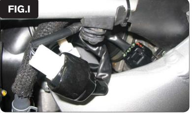
14 Attach the connectors from the PCFC to the stock TPS connector and the stock wiring harness as shown in Figure I.
