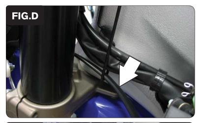
Route the PCFC harness through the cable guide on the left hand side of the frame as shown in Figure D.
