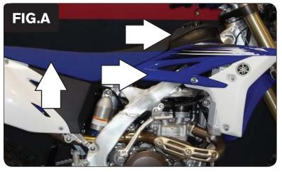
1 Remove the seat, the radiator side covers, and the fuel tank as shown in Figure A.
