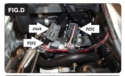
Attach the connectors from the PCFC wiring harness to the fuel injector and the stock wiring harness as shown in Figure D.
