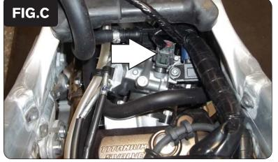
5 Locate and unplug the stock wiring harness from the fuel injector on top of the bike's throttle body as shown in Figure C.
