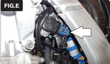
7 Locate and unplug the stock wiring harness from the bike's Throttle Position Sensor (TPS) as shown in Figure E.
