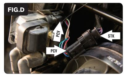
5 Plug the PCV wiring harness in-line of the Ignition Coil and the stock wiring harness (Fig. D).
