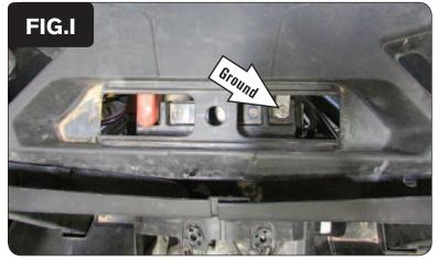
Route the PCV ground wire (single BLACK wire with the small ring lug) to the battery (behind the seats), and secure the ring lug to the negative terminal of the vehicle's battery (Fig. I).
