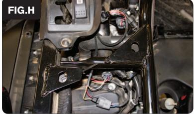
11 Plug the PCV wiring harness in-line of the Fuel Injectors and the stock wiring harness (Fig. H).
