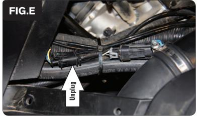
Route the PCV wiring harness branch with the pair of 2 pin connectors with BROWN colored wires downward to the Vehicle's Crank Position Sensor connectors.
