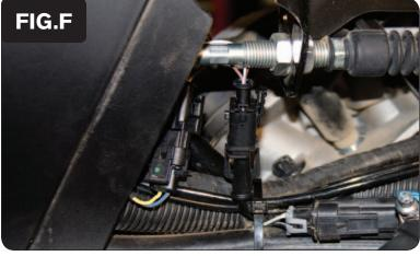
Plug the PCV wiring harness in-line of the stock Crank Position Sensor connectors (Fig. F).
