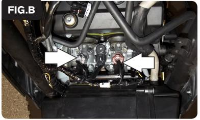
3 Unplug the stock harness from the fuel injectors (Fig. B)
