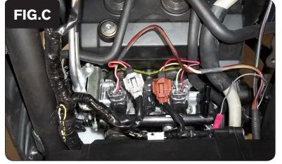
4 Plug the PCFC in-line of the stock injectors and wiring harness (Fig. C)
